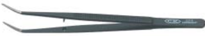
▲ 2315 C UNIVERSAL TWEEZERS 150 mm 6" Tip width 1.5 mm. Fine blunt points, bent 15 mm. Finely milled inside. With guide pin. Polished and black coated up to 10 mm from points. Serrated grips.
