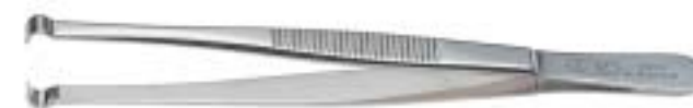
▲ 2303 C POSITIONING TWEEZERS 140 mm 5.1/2" Tip width 5 mm, for horizontal devices of minimum 5 mm Ø. Polished and fine nickel plated. Serrated grips.
