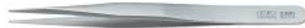
▲ 2386 SMD POSITIONING TWEEZERS TYPE SM116.SA 120 mm 4.3/4" For vertical holding and positioning of cylindrical devices from 1 mm Ø. Grooved, straight tips.
