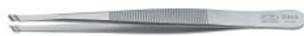
▲ 2353 SMD POSITIONING TWEEZERS TYPE 579.SA 115 mm 4.1/2" For holding, positioning and desoldering vertical and horizontal cylindrical devices up to 2 mm Ø. Tips round inside. Serrated grips.
