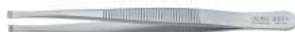
▲ 2351 SMD POSITIONING TWEEZERS TYPE 582.SA 115 mm 4.1/2" For holding, positioning and desoldering horizontal cylindrical devices up to 1 mm Ø. Tips round inside. Serrated grips.
