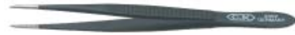
▲ 2302 C UNIVERSAL TWEEZERS 115 mm 4.1/2" Tip width 1 mm. Fine blunt points, finely milled inside. Polished and black coated up to 10 mm from points. Serrated grips.
